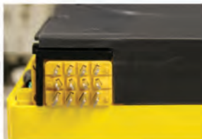
⑧ Make sure connector pins line up with socket on baseplate. If not remove, rotate 180° and repeat step 7.
