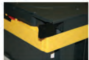
⑥ Place insert plate on opposite side. "L" piece must always be on top.
