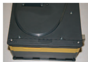
⑪ Place strip back over cable.
